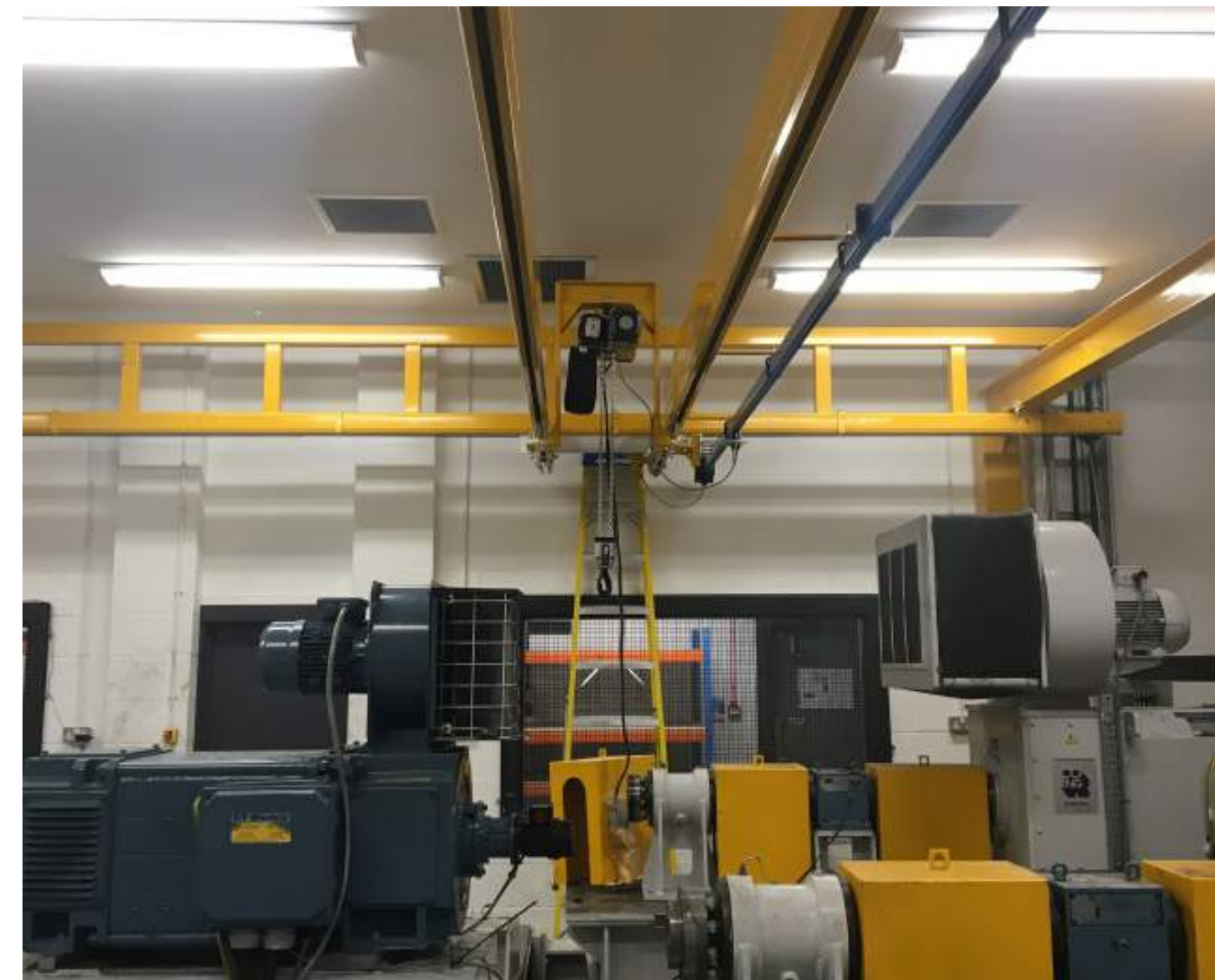
Ultra low headroom crane system with girders (bridges) upraised between the runway tracks
