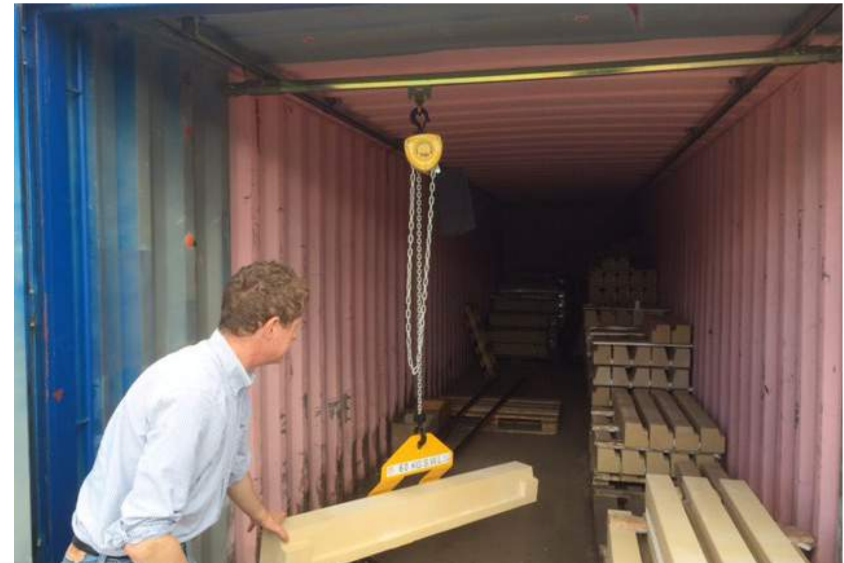
Crane installed in container for loading & positioning goods in pallets
